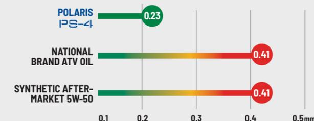
ASTM D4172. In 3rd party testing against 9 competitive products Polaris had 40% or better wear protection compared to all of the tested products. Numbers represent mm of wear scarring measured. Test measures wear at contact points, wear scar is measured for its length and width (in units of mm). Lower wear numbers mean better wear protection and friction reduction.
