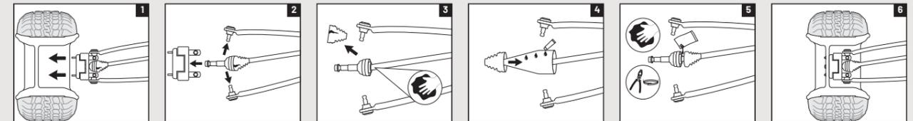
1 Remove wheel and axle nut.
