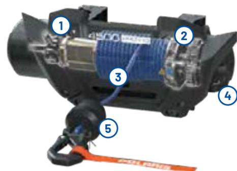
1 **Sealed permanent magnet motor**
